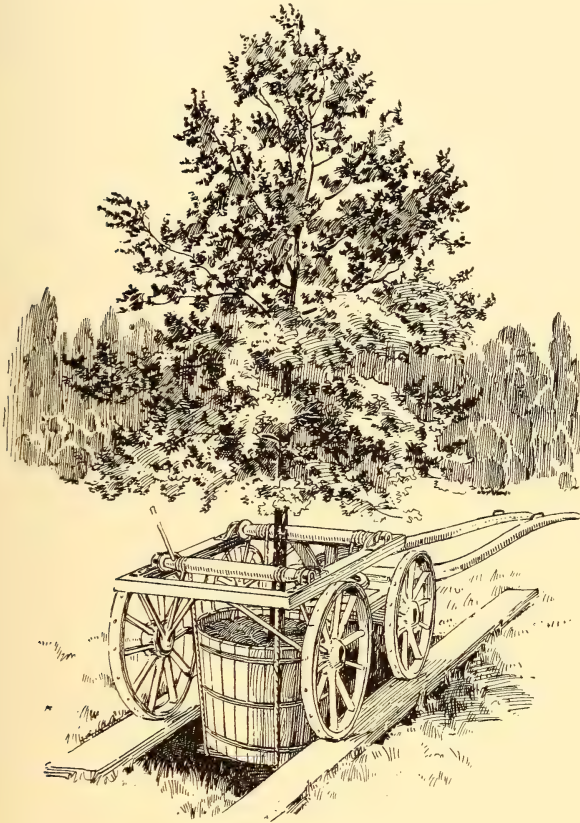
Figs. 319 and 320.—View and Side Elevation of Transplanting Machine for Trees of large size. The mass is raised by means of iron crowbars which fit into sockets in the rollers around which the lifting-ropes are wound.
